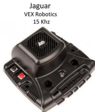
Jaguar VEX Robotics 15 KHz Interface: PWM CAN (CAN = Controller Area Network) WPILib Class: Jaguar
