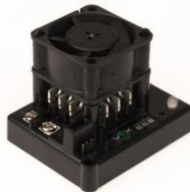
Victor 888/884 VEX Robotics 1 KHz
